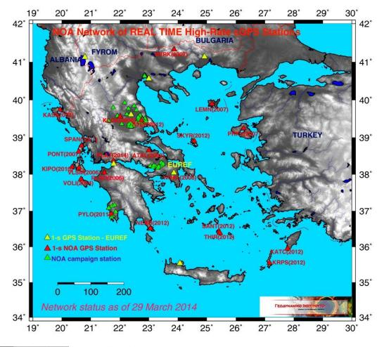
following the EUREF (Regional Reference Frame Sub-*Commission for Europe*) Permanent Network standards 22 stations at 1-s 24/7 12 stations co-located at 1-10m with seismometers and strong-motion sensors 55 benchmarks
