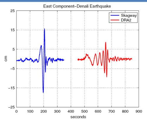
**Fig. 2** East component GPS displacement records for a Skagway site and DRA2. These GPS receivers were located over 700 and 2,200 km, respectively, from the Denali epicenter. The difference in arrival times for the seismic displacements reflects the additional time it took the surface waves to travel the 1,500 km between Skagway and DRA2
